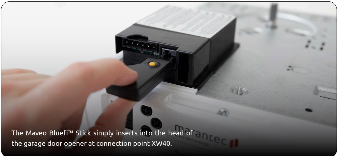
The Maveo BlueFi™ Stick simply inserts into the head of the garage door opener at connection point XW40.
